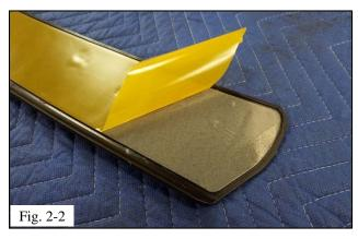
(d) While keeping the bumper protector aligned, lower the part in place. Pull small sections of the backing (Fig. 2-2) while pressing the part onto the vehicle until you have removed all of the backing and the part is secure.
