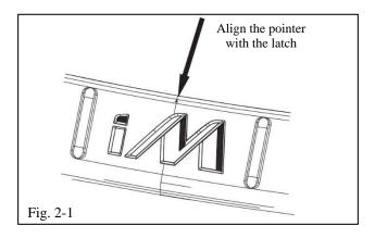
(c) Hold the bumper protector about ½" above the surface of the bumper and align the center indicator (pointer) on the bumper protector to the center of the latch on the rear lift gate (Fig. 2-1).
